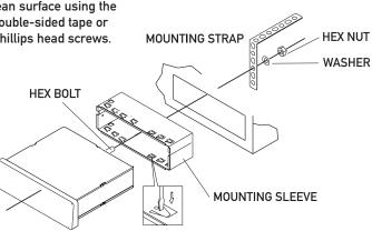
TYPICAL FRONT-LOAD DIN MOUNTING METHOD
